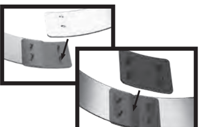
4. Stand 2 wall sections end to end & align holes with posts on outer wall clip. Place inner wall clip on other side & snap together.
