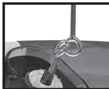
8. Maintaining a firm hold on the sides, attach the paint pot to the string hook. DO NOT LET THE POT HANG FROM THE STRING UNTIL YOU ARE READY FOR PAINT TO COME OUT.
